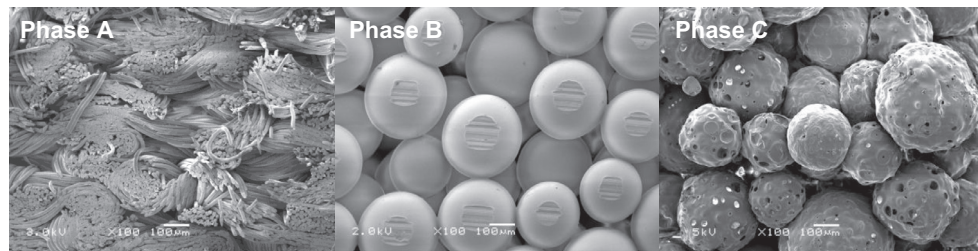
Fig. 2. Microstructure of phases A, B, and C of the tri-phasic scaffold.
